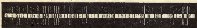
FIG. 267. — Showing the Coincidence of the Bright Lines of the Spectrum of Iron with Some of the Dark Lines of the Solar Spectrum.
